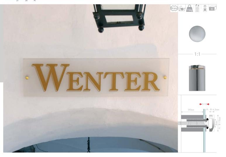
**EN economical, for pre-assembly.** in the workshop signs and panels can be pre-assembled and fastened between wall spacer and centerpiece. on site mark the wall holes and place the dowels. mount the sign to the wall and press on the deco-head. for easy mounting: screw can move slightly in the spacer allowing to compensate defiance of the boreholes in the wall.
