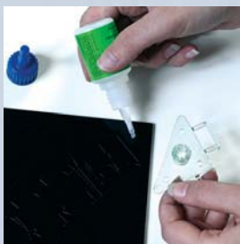
spacers can be mounted to the sign with appropriate glue
