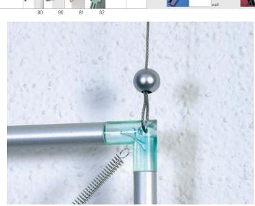
**EN loop clamp for cable.** slide through steel cable or nylon thread forming a loop and fast it with allen screw. <u>mounting</u>: loop clamp for cable, screw system. <u>material</u>: chrome-plated brass. <u>cable thickness</u>: max. Ø2mm.
