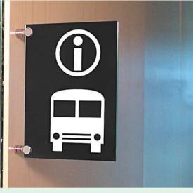
**EN variable panel support for wall/ceiling.** for wall- or ceilingmounted flagsigns. adjustable to panel thickness. fixing of the panel with allen screws. <u>mounting:</u> panel support for wall/ceiling, variable, screw system. <u>material:</u> silver- or chrome-plated brass. <u>panel thickness:</u> max 10mm. <u>wall distance:</u> 15mm. <u>panel hole:</u> Ø>4mm.
